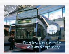
The vehicles on the extensive King Long stand included an airport apron bus that was 13.83 metres long and 3.0 metres wide. It was powered by a Cummins ISBe220 engine and had a front-wheel drive layout. This large bus had capacity for 140 passengers, with access doors on both sides. Zhengzhou Yutong showed the first open-top double deck bus built in China, for city sightseeing. It had an overall length of 11.975 metres on two axles and had two staircases.
